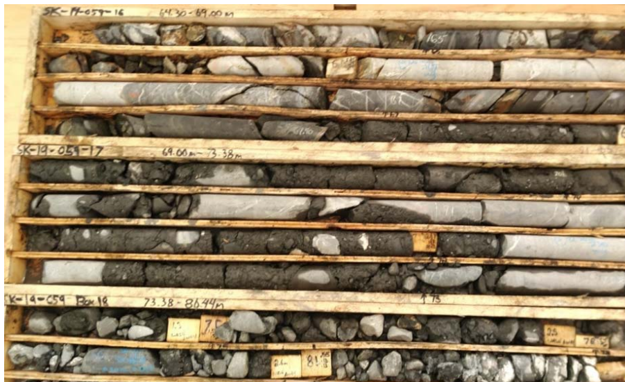
Figure 16-4: Contact Mudstone Typical Drill Core Intercept
