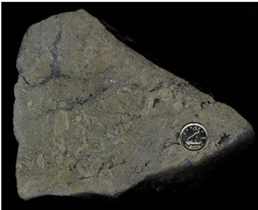
Figure 7-7: HW Zone – Massive strata-bound sulphide lenses within the hanging wall mudstone (Gale et al., 2004)
