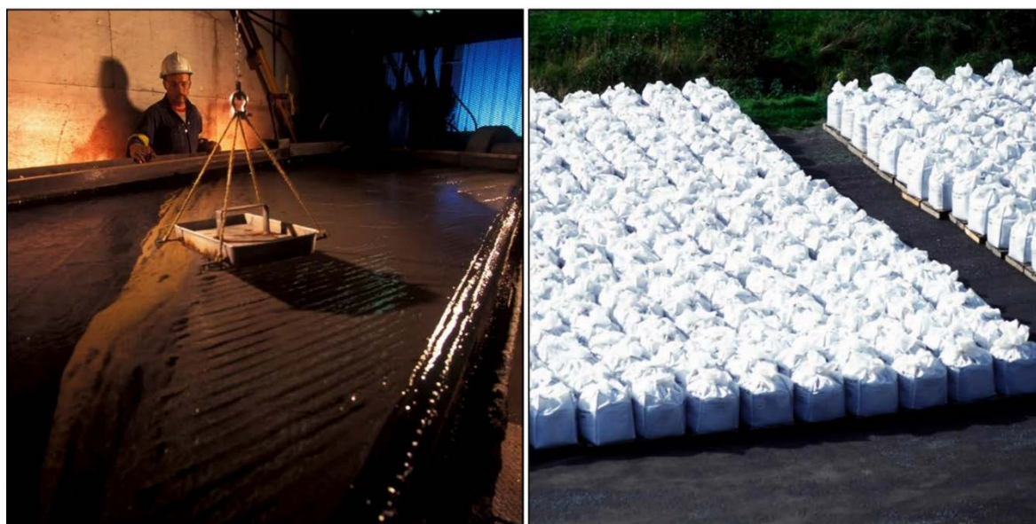
Figure 6-2: Recovery of gold from historical Snip Mine, circa 1998. (Left) Free gold on shaker table, (Right) Heavy bags of sulphide concentrate
