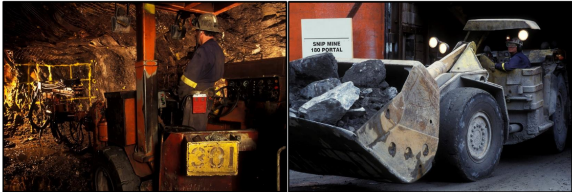
Figure 6-3: Mining at the historical Snip Mine, circa 1998. (Left) Jumbo mechanized drilling, (Right) scoop tram exiting 180 level portal
